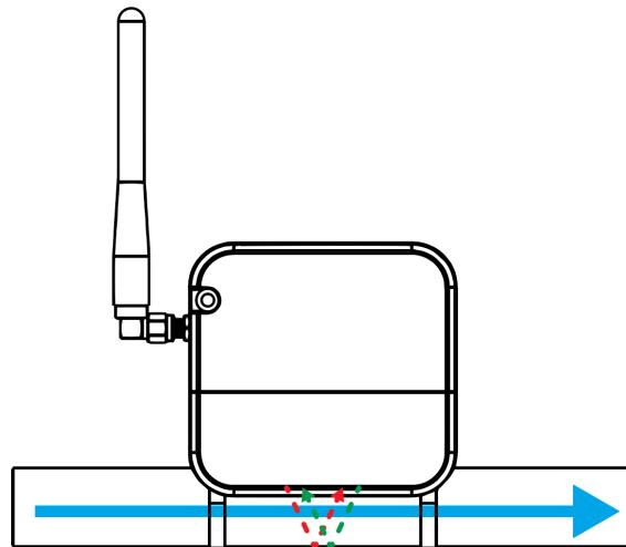
The CubicMeter measures the flow of water with the use of ultrasonic waves and the “differential time of flight” method.
